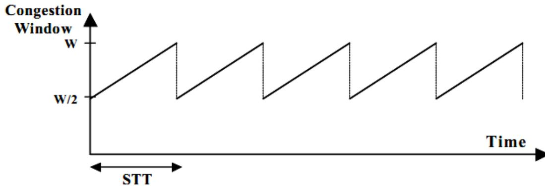
The picture above shows the famous TCP sawtooth behavior. We are assuming that fast retransmit and fast recovery always work, i.e. there are no timeouts and there is exactly one packet lost at the end of each “tooth”. We are assuming that the flow control window is large and that the sender always has data to send, i.e. throughput will be determined by TCP congestion control.
